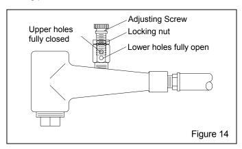
**5.3.3** If pulsation occurs in the media hose, either media is damp and caked, or not enough air is entering the media stream. While blasting, loosen the locking nut and slowly turn the adjusting screw out (counterclockwise when viewed from the top) until the media flows smoothly.
