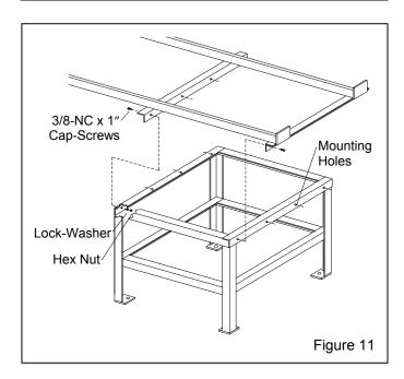
**3.4.3.3** Push the track assembly to its final position; the end support bracket should be against the inside cabinet wall, and the middle bracket against the outside wall under the door opening, as shown in Figure 12.
