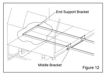
**3.4.3.4** Match drill 9/32" holes through the cabinet wall, at the two holes in the end support bracket. If necessary, mark the hole locations and move the track for drilling.
