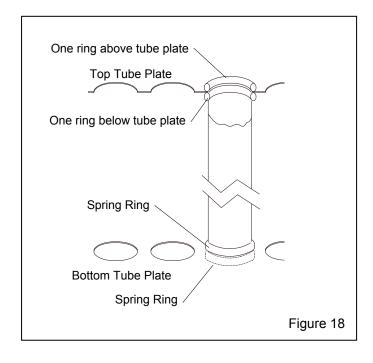
**7.6.2** The tubular filter is held firmly by a spring ring above and below the perimeter of the hole in the plate. The other end of the filter is similarly installed in the lower plate. The filters fit tight to prevent dust leakage. To ensure a tight seal, some force may be required by the installer. Check for proper seating at both ends, and remove any twist in the tube before proceeding to the next filter.
